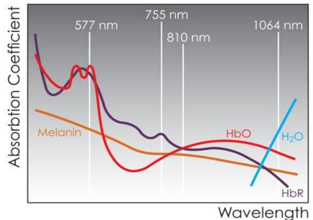
**Fig. 6. Absorption characteristics of green and infrared beam Laser<sup>(27)</sup>**
