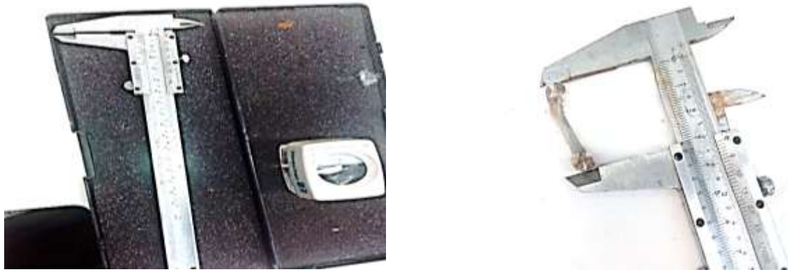
Figure 4. Vernier caliper used for measuring the femoral bone length and thickness
